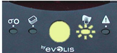
If the printer is not cleaned, the light will remain illuminated and will then start flashing after an 100 additional cards have been printed. In this event, immediately stop the work in progress and proceed with the cleaning.
