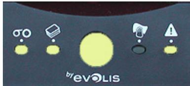
Control panel display - MECHANICAL PROBLEM - Work is interrupted.
